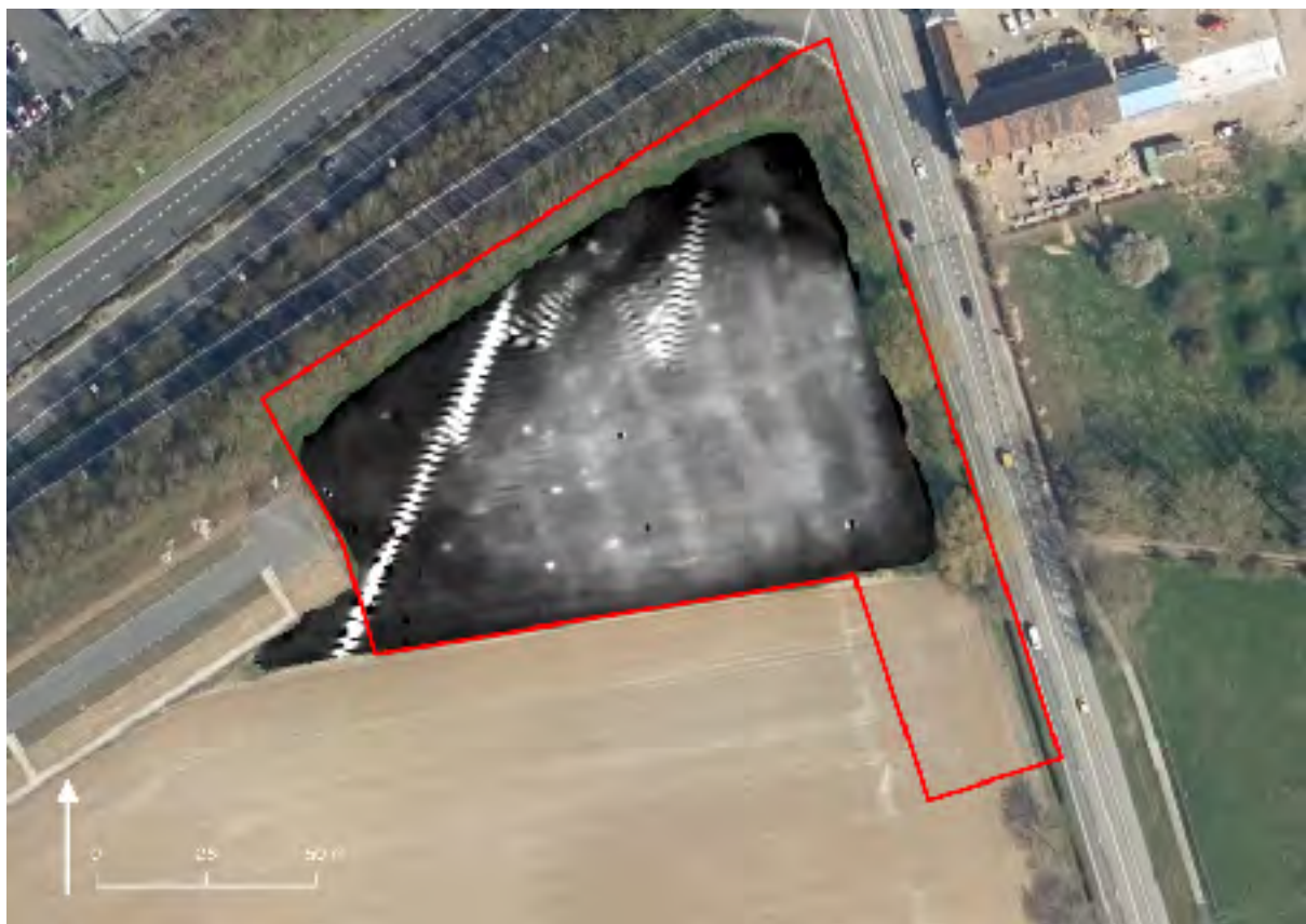
Fig. 5. Electrical conductivity survey of MSJ, showing linear features
